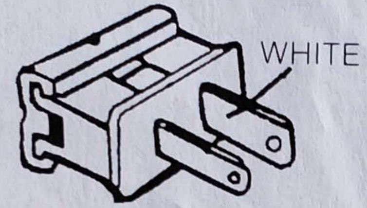
1. This is a polarized plug. One blade is wider and marked WHITE. This blade must be connected to ribbed side of wire.
